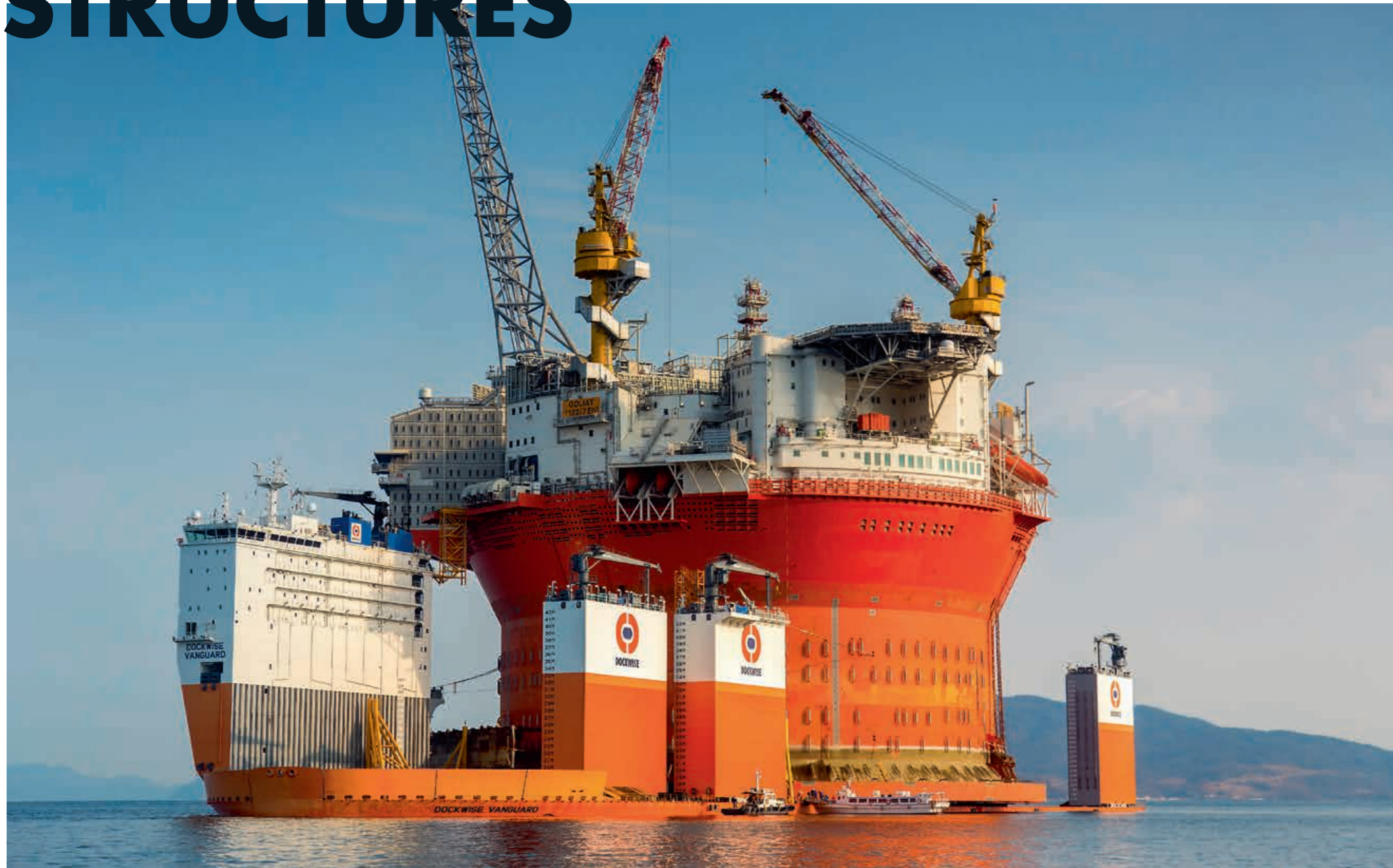
SOUTH KOREA – NORWAY Transport of the Goliat FPSO, with a diameter of 107 meters, onboard the Vanguard.
