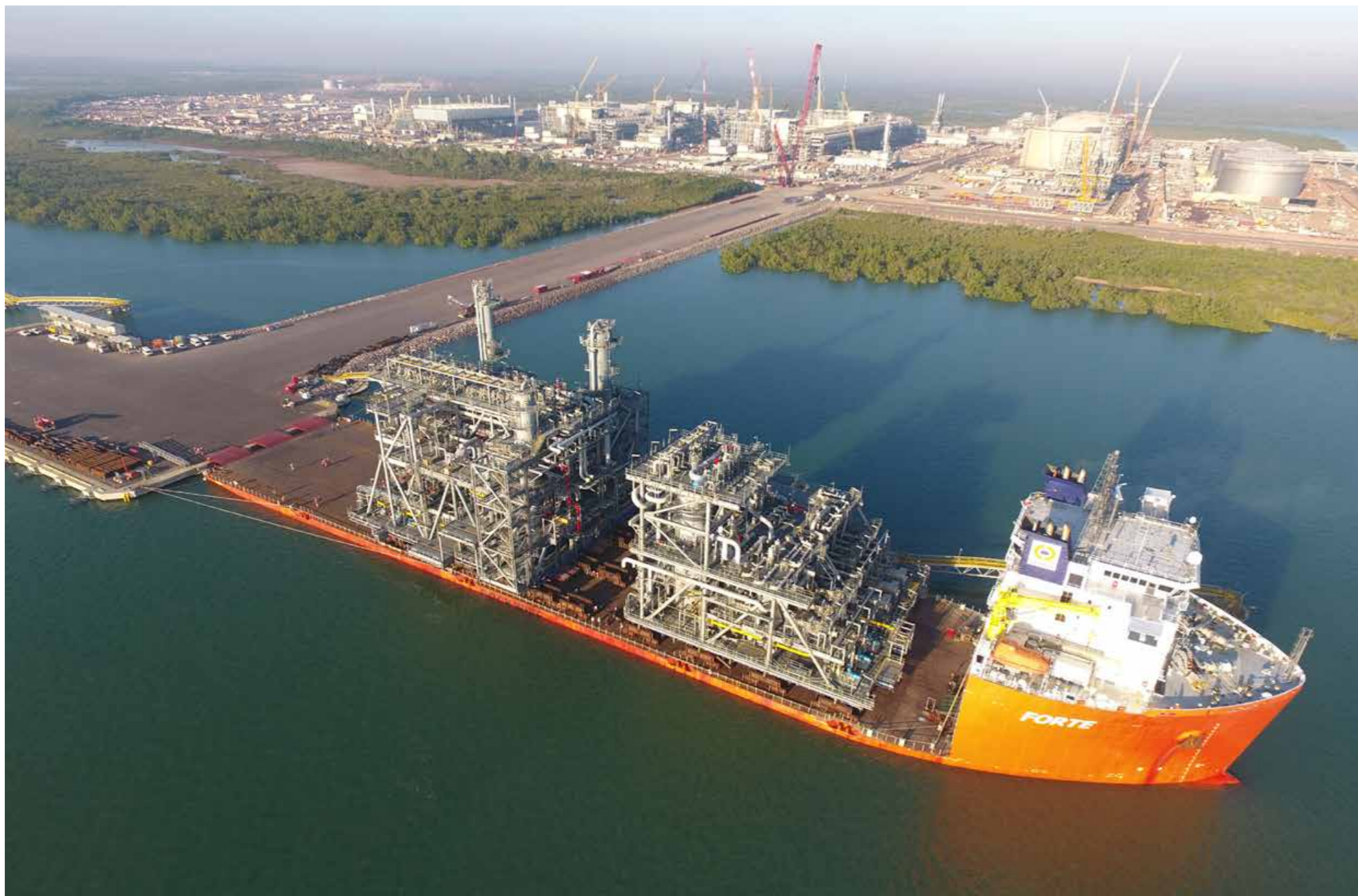
DARWIN, AUSTRALIA Logistical management services for the Ichthys LNG project, including 19 transports of modules with a.o. the Forte from different fabrication yards to the LNG plant in Darwin.
