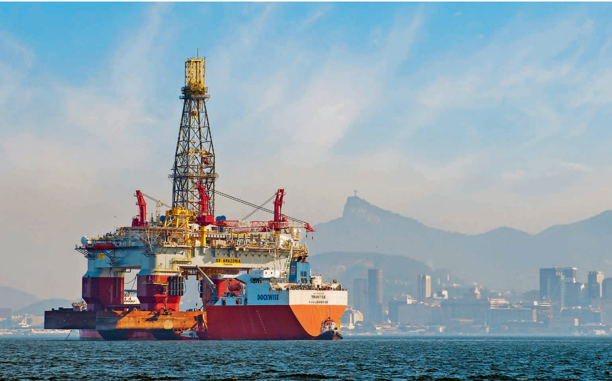
CHINA - BRAZIL The semi-submersible drilling rig SS Amazonia onboard the Trustee. Draft restrictions required removing the thrusters in order to transport the rig.
