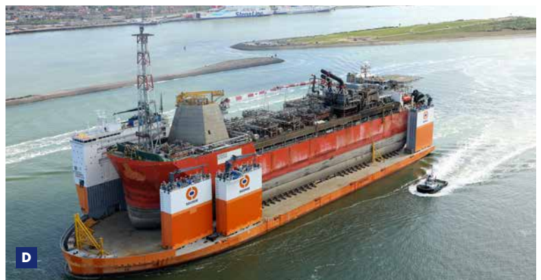
C The Dockwise Vanguard submerged D FPSO Armada Intrepid onboard the Dockwise Vanguard
