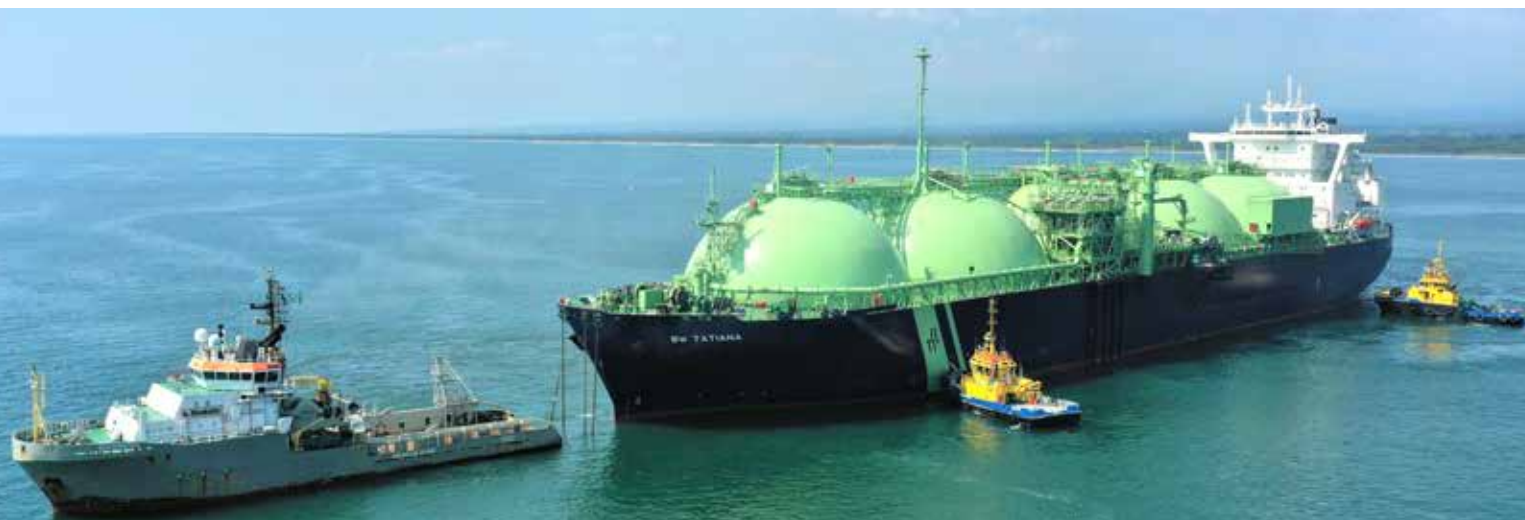
Hook-up of a Floating Storage and Regasification Unit by the anchor handling tug supply vessel Sovereign off the coast of El Salvador
