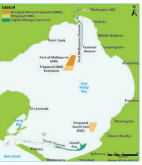
Figure 3. Scope of the dredging works.
